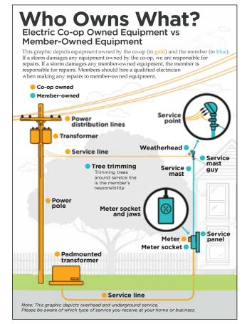
the trench and the conduit for this installation. The cooperative installs and owns the service wire from the transformer to the meter base.
