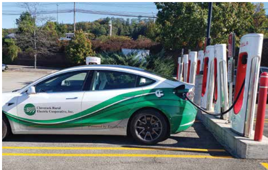
PIT STOP: Claverack's Tesla electric vehicle fuels up at a level 3 fast-charging station near Rochester, N.Y. The "fill-up" added 173 miles of range at a cost of $14.62.
